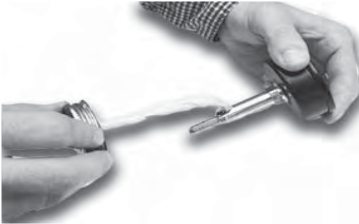
Figure 7 - Apply Pipe Sealant On Shaft of Gauge
